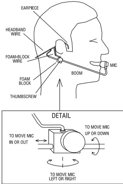
2. Loosen (just a little) the thumbscrew located on the outside of the foam block, part way back on the boom. This allows the boom to slide in and out, and to rotate left and right.
