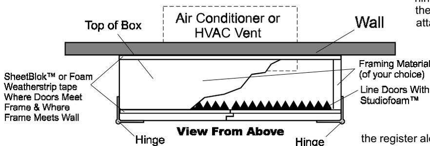
Another trick if you're retrofitting a noisy register cover, especially one that's on a wall instead of a floor—Build a wide box that covers the register & then extends away from the register along the adjoining wall. This box (more like a chute really) should be lined with lightly-painted 1" duct board to quiet internal air movement. At the
