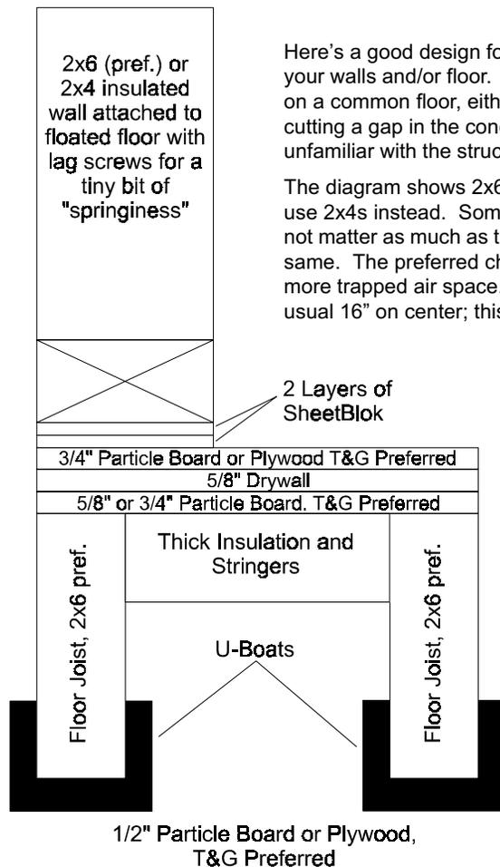
Here's a good design for those of you who have the vertical space to spare and need to float your walls and/or floor. This is perfect for when a studio and control room are both going to rest on a common floor, either wooden or a concrete slab. If yours is concrete, consider (carefully) cutting a gap in the concrete between the two rooms first, then proceeding as follows. If you're unfamiliar with the structural ramifications of doing this, please consult a local expert.
