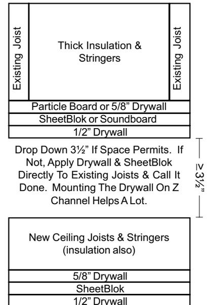
*Diagram showing the correct way to layer your ceiling material, whether you're framing a lowered false ceiling or just applying more layers to your existing.*
